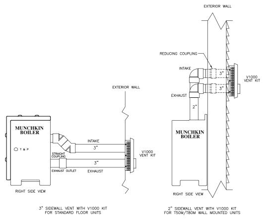
\*\*IMPORTANT NOTE: All vent pipes must be glued, properly supported and the exhaust must be pitched a minimum of a 1/4" per foot back to the heater (to allow drainage of condensate).
